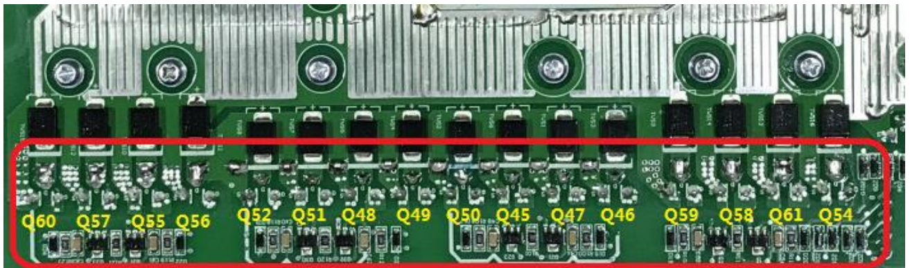
Figure 5.4.2 DC-DC Converter/ MOSFET
