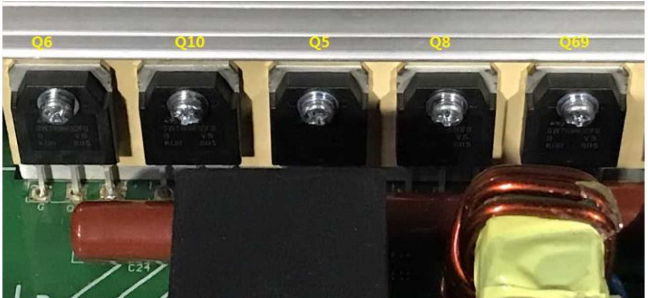
Figure 5.4.5 DC-AC Inverter/ IGBT
